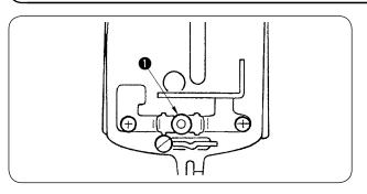
If the formation of seams at the start of sewing is failed and the seams are formed on the way even when the thread pull-off lever is adjusted, turn thumb nut (double nut) to decrease the thread tension.
