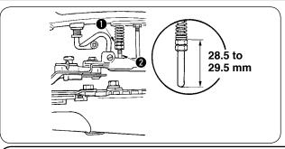
The standard work pressing force is by providing a 28.5 to 29.5 mm between the top end of nut ① and the bottom end of pressure adjusting bar ②.
