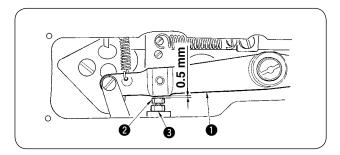
Provide a 0.5 mm clearance between the end face of button clamp lifting lever 1 and adjusting screw 2 at the stop-motion position (refer to "3-14 Adjusting the position of the stop-motion", p.8) and tighten with adjusting screw nut 3.
