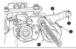
In the state of 16 stitches, stitch number adjusting gear roller 2 which is attached to the large gear 5 comes to the lower side, assemble stitch number adjusting lever 4 (supplied as accessories) using hinge screw 3 (supplied as accessories).
