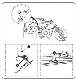
Loosen screws and adjust so that a clearance of 1 to 1.5 mm is provided between the needle and the knot tying plate when the roller of the knottying arm gets on the outmost periphery of the knottying notch.
