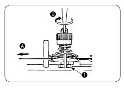
Turn the needle driving pulley as you draw the thread in the direction of arrow mark (a) and you will find a point at which the tension discs on the tension post No. 2 release the thread. At this moment, the standard distance from the top end of the needle bar bushing (upper) to the top end of the needle bar is 44 to 47 mm (in case of the needle of TQ X 7, 54 to 57 mm).
