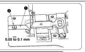
Loosen screw 2 and provide a 0.05 to 0.1 mm clearance between the needle guide 1 and the needle by moving the needle guide 1 to the left or the right when the needle is in the lowest position.
