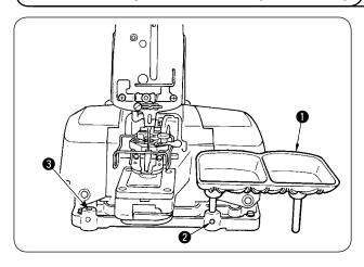
Insert the posts of button tray ① in hole on the right of the machine sub-base and tighten each setscrew ②. If it is difficult for the operator to pick up the buttons on the right side, change it to hole ③ on the left side.
