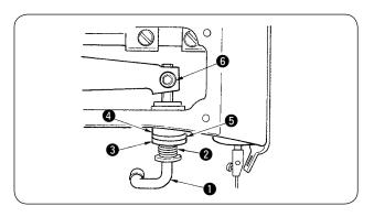
Put moving knife push-back spring ②, stop-motion rubber cushion washer ③, stop-motion rubber cushion ④ and stop-motion rubber cushion washer ⑤, in this order, to L-shaped lifting rod ①. Make the jaw of the machine arm come into close contact with the end face of the stop-motion rubber cushion washer at the stop-motion position (refer to "3-14 Adjusting the position of the stop-motion", p.8) and set the L-shaped lifting rod without a play. Then tighten it with screw ⑥.
