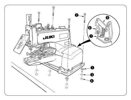
Put rubber cushion ① on the table, place the machine head on the rubber cushion and fix it to the table using screws ②, plain washers ③ and nuts ④. Attach "S" chain hook ⑥ and chain
