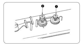
Tension post No. 1 is used to adjust the thread tension to sew on the button and a relatively low tension will be enough. Tension post No. 2 is used to adjust the thread tension applied to the root of the button sewing stitches. This tension must be determined according to the type of thread, fabric and thickness of the button and must be higher than that of tension post No. 1 Turn the tension nuts clockwise to increase or counterclockwise to reduce the thread tension.
