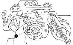
To make 8 stitches, loosen stitch number adjusting screw **1** and fix it to the position as shown in the illustration.
