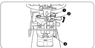
When clamp screw 1 is loosened in the state of stop-motion, button clamp jaw levers 3 opens/closes with button clamp stop lever 2. Set a button to the correct position and fix button clamp stop lever 2 at the position where taking in and out of the button is easily performed with clamp screw 1.
