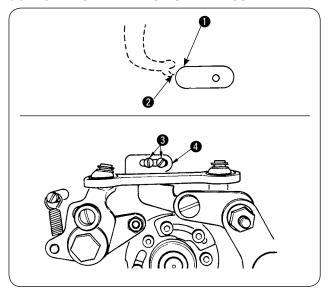
When starting the sewing machine and the roller of knot-tying arm does not come into contact with the knot-tying notch, loosen screws 3 and adjust with stopper 4 so that outside periphery 1 of the needle hole almost aligns with top end 2 of the knot-tying plate.
