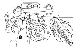
When stitch number adjusting screw ① being set for "8 stitches" has arrived at the left end, loosen stitch number adjusting screw ① and fix it to the position as shown in the illustration.
