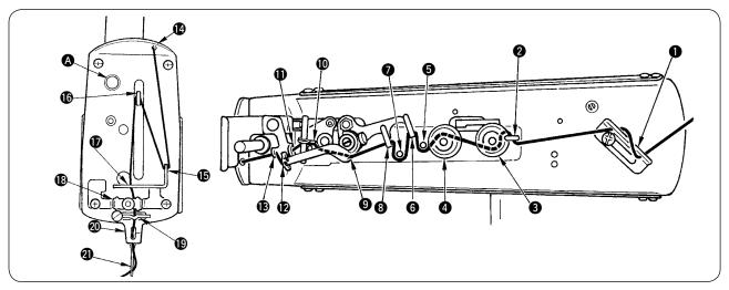
Thread the machine head in the order of **1** to **2** as shown in the illustration given above. Then, pass the thread through the needle eye from the front for approximately 60 to 70 mm as you depress nipper releasing knurled thumb nut **3**.
