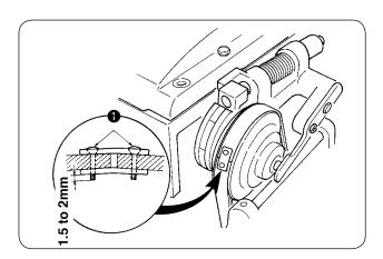
Tighten connecting screws • of the belt so that the screws protrude approximately 1.5 to 2 mm from the reverse side as the standard.
